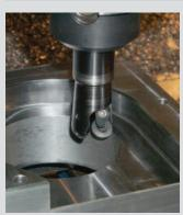
Larger diameter hole making can be quick and easy when a Toroid Cutter is used in combination with helical interpolation. This technique resembles thread milling in that all three axes (X, Y and Z) are in motion simultaneously. It differs from thread milling in that the tool is introduced into the material without a start hole of any kind. The tool simply is positioned at the inside diameter of the hole
