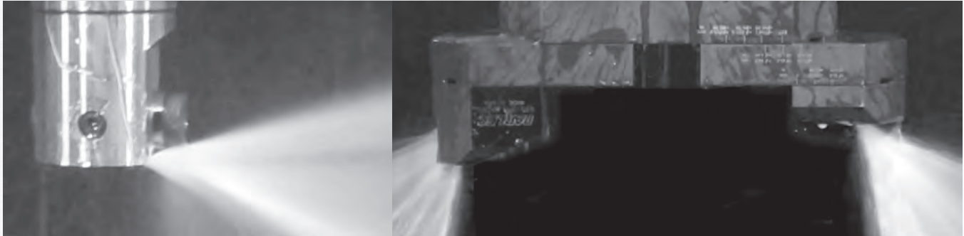
Tool life and chip form are maximized by directed high pressure coolant
